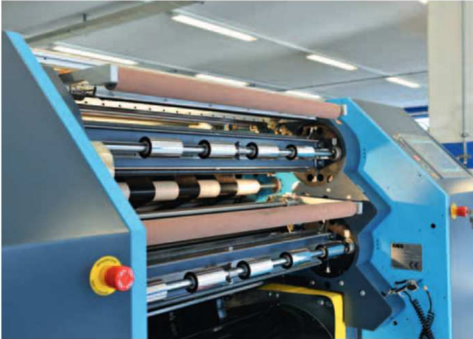
A combination of a slitting and winding machine and a turret winder with automatic leader applicator
